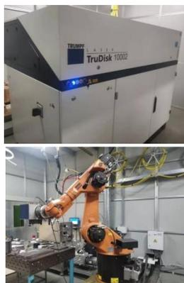
(a) laser structure (b) six degree of freedom robotic arm
