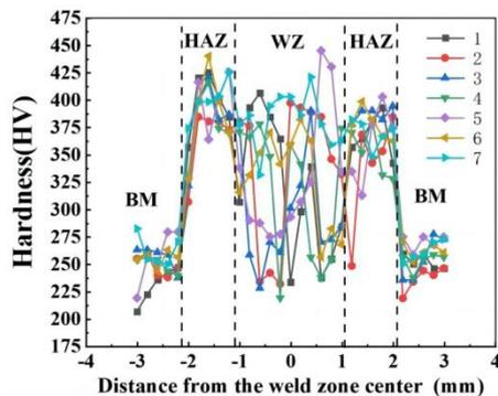
Fig.7 Microhardness of welded joints under different scanning paths
