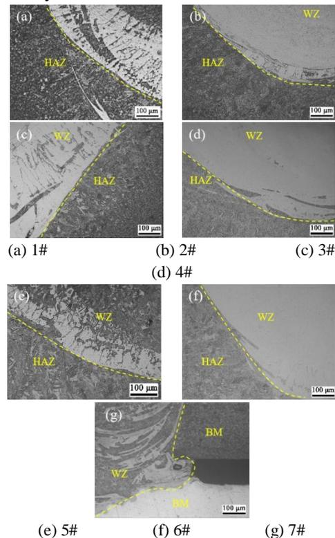
Fig.6 Bottom structure of different welded joints
