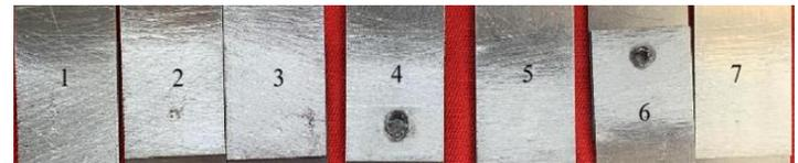
Fig.4 Weld morphology of different spot welded joints
