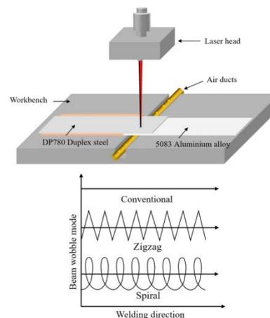
(a) Overlap welding schematic diagram
