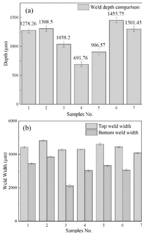
Fig.5 Weld size of different specimens
