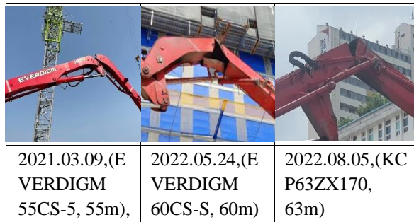
Fig. 1. Accident status during concrete pouring
