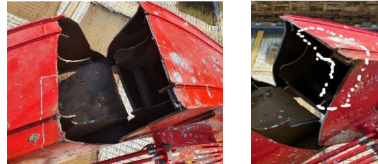
Fig. 3. A sectional photograph of the pump car boom breakage of company D社 (death 2).
