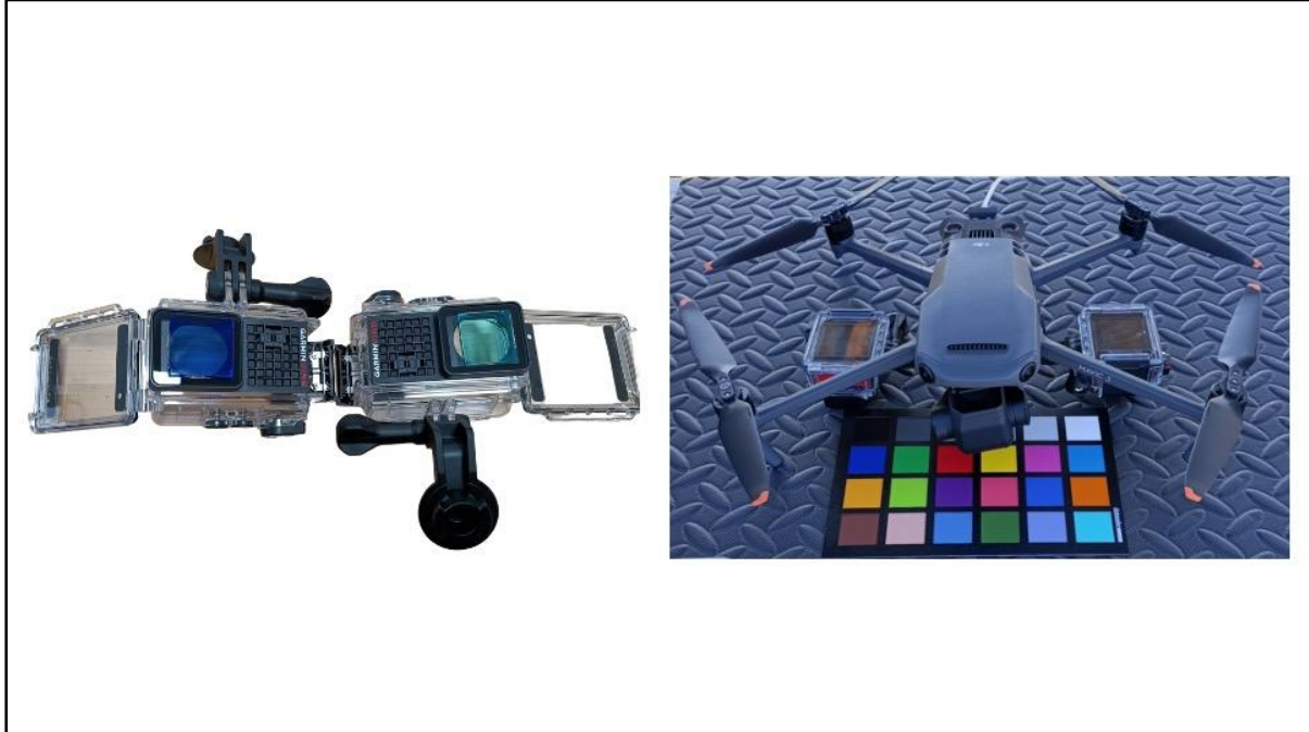
Figure 1: Customization of the drone: on the left, the two GPS-enhanced micro-cameras with two multiband-pass optical filters and their integration with a DJI Mavic 3, on the right.
