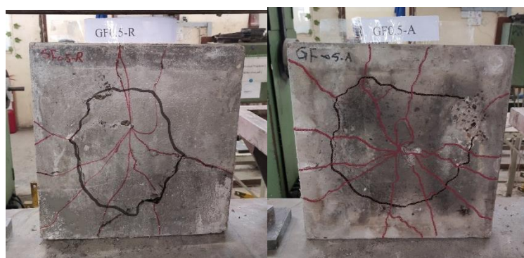
Fig. 16 crack pattern and punching perimeters of normal strength concrete
