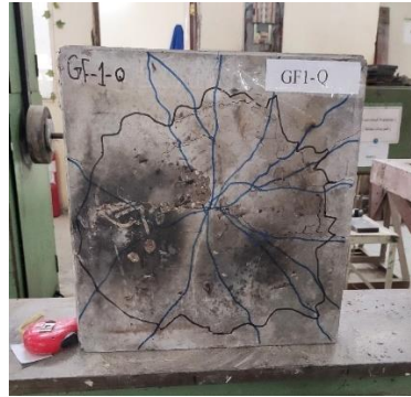
Fig.18 Crack Pattern and Punching Perimeters of 1.0 % Glass Fiber Concrete
