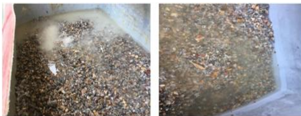
Fig. (4) RCA Treatment with Acid
