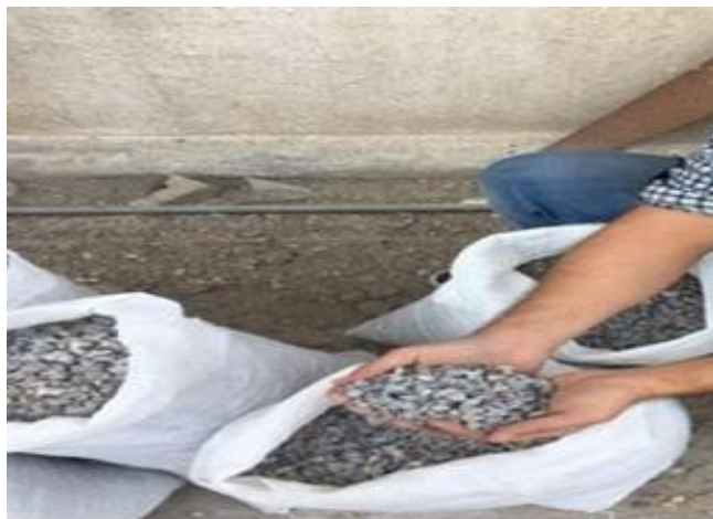
Fig. (3) RCA after crushing and sieving
