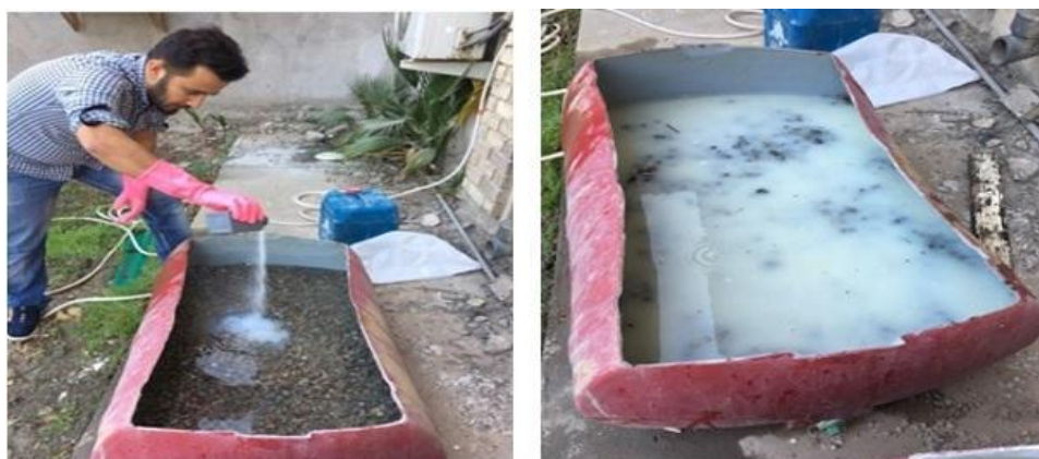
Fig. (5) Coating the RCA in sodium metasilicate pentahydrate
