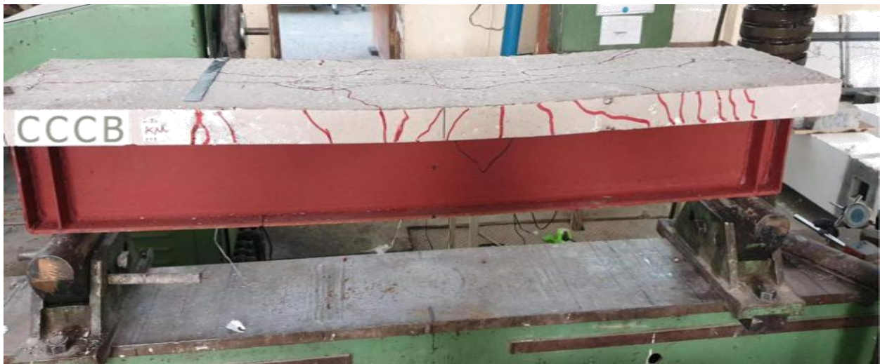
Figure 9: Composite beam CCCB at failure stage
