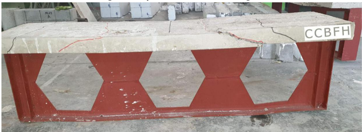
Figure 10: Composite castellated beam CCBFH at failure stage
