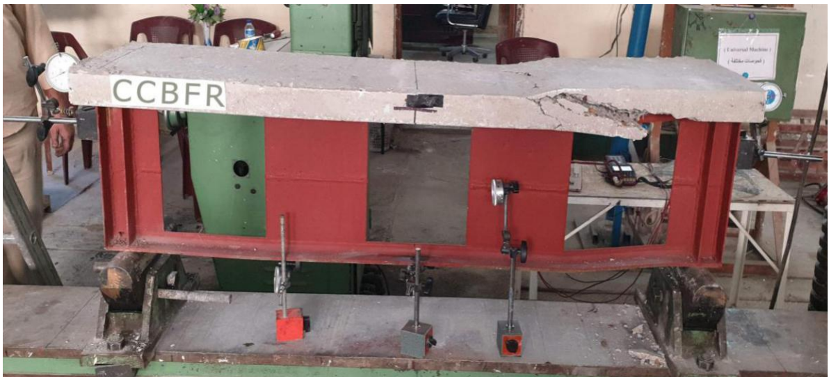
Figure 12: Composite castellated beam CCBFR at failure stage
