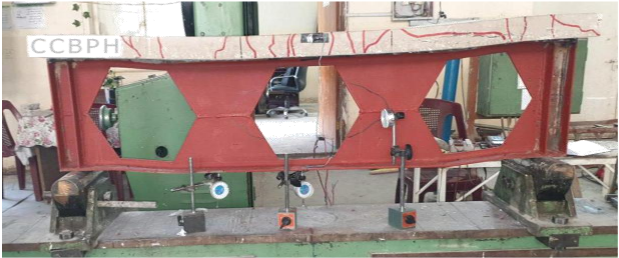
Figure 11: Composite castellated beam CCBPH at failure stage
