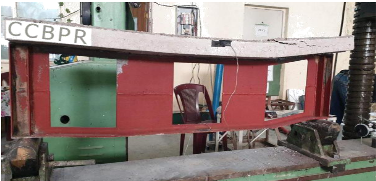
Figure 13: Composite castellated beam CCBPR at failure stage
