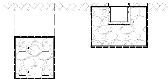
Fig.4 Typical structure sketch of seepage pipe
