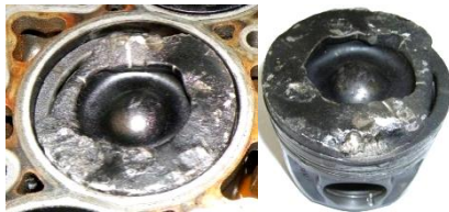
Fig.1 Piston Top Melting and Deformation
