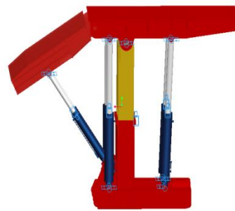
Fig.1 The model and constraints of hydraulic support
