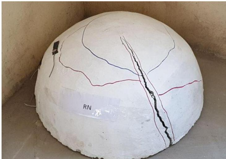
**Figure (13) Crack Pattern of Specimen NR**
