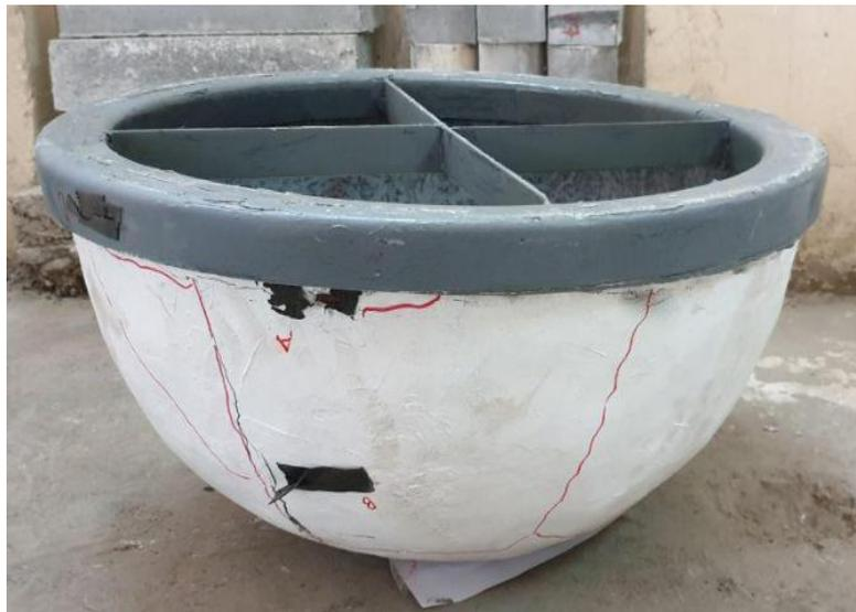
**Figure (1) Dome Braced with Steel Rib**
