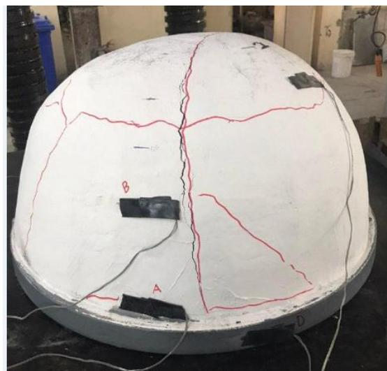
**Plate (17) Crack Pattern of
