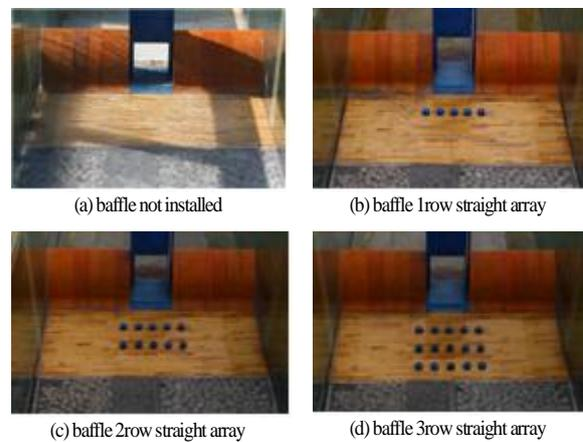
**Figure 5. Arrangement conditions**
