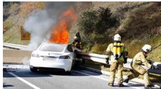
figure 2 Battery combustion caused by vehicle collision
