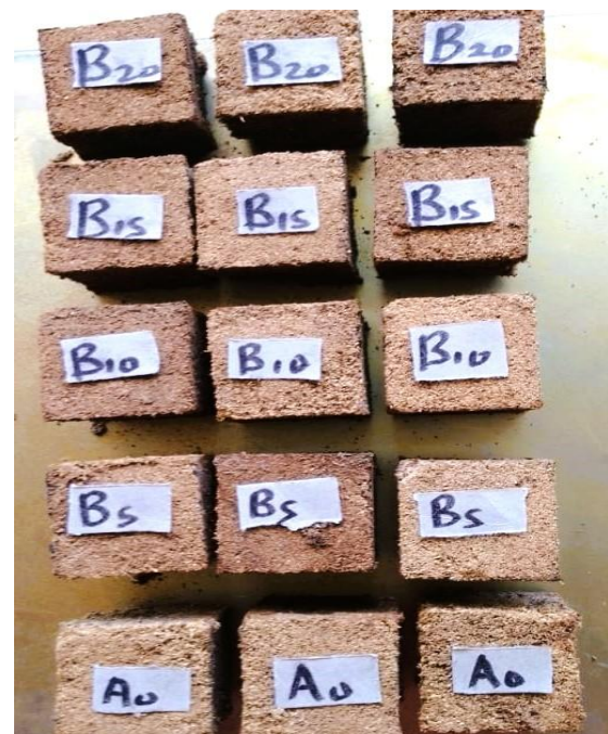
Fig. 4 Cubes being cured
