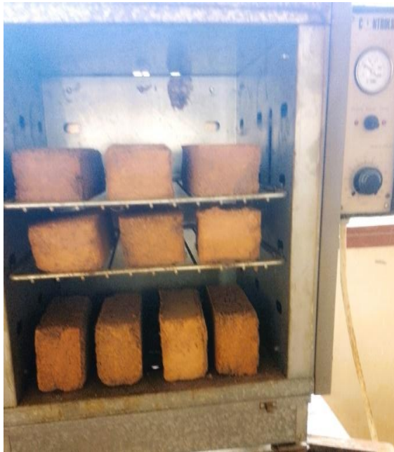
Fig. 5 Burning of bricks in an electric oven
