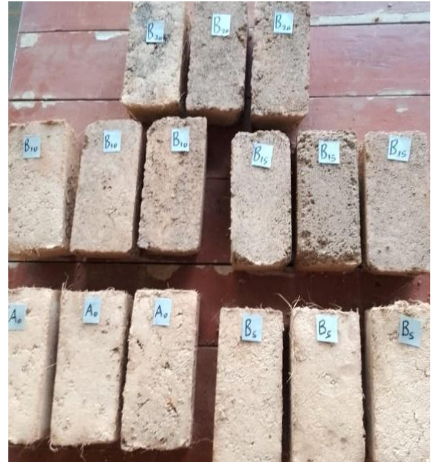
Fig. 3 Bricks being cured
